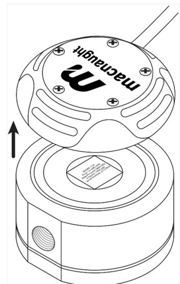
Place pulse cap onto the body and rotate 90° clockwise to reassemble
