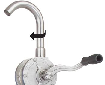
2. Attach the crank to the shaft on the pump and tighten bolt ensuring that the bolt is aligned correctly into the depression on the shaft.
