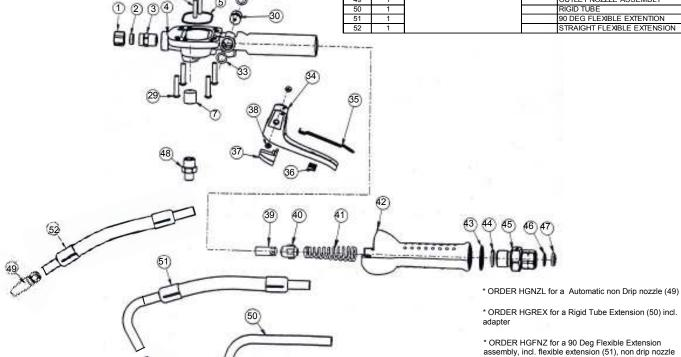
\* ORDER HGFNZ for a 90 Deg Flexible Extension assembly, incl. flexible extension (51), non drip nozzle
